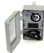
Each unit includes a UL Approved Control Panel complete with Class A Human Rated GFCI Protection, 24 Hour Mechanical Timer, and Photo Eye for Optional Light Kit. NEMA Type 3r nonmetallic enclosure.
